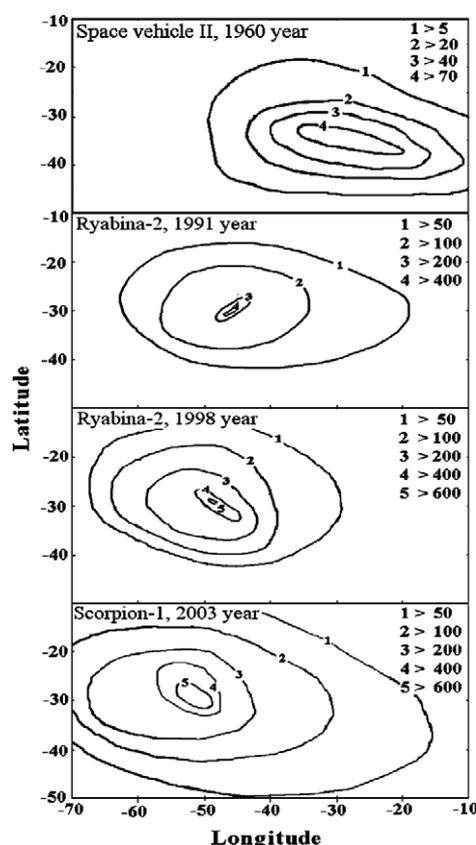
Fig. 2. Proton fluxes intensity isolines reconstructed from the observations of setups Space vehicle II in 1960 (the flux is given in relative units), Ryabina-2 in 1991, 1998 and Scorpion-1 in 2003 (count rate levels are shown, s<sup>-1</sup>).
